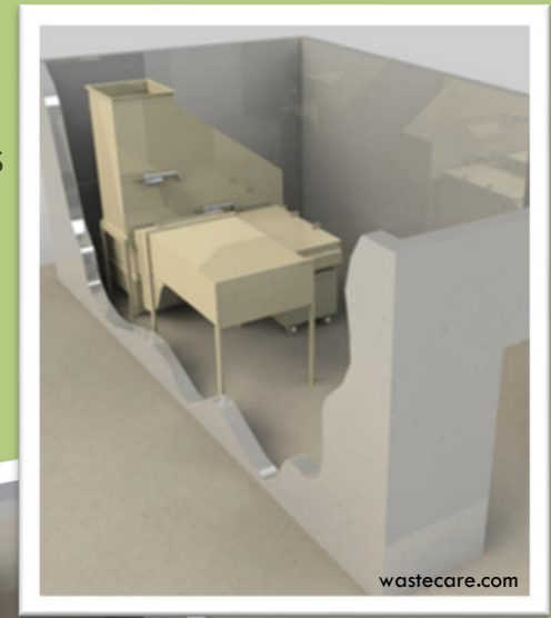
3-D renderings of an installed chute system
